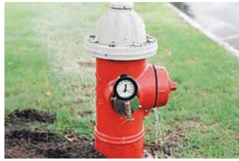
Flushing of Residual Hydrant (left) and Attachment of Test Equipment (right).
