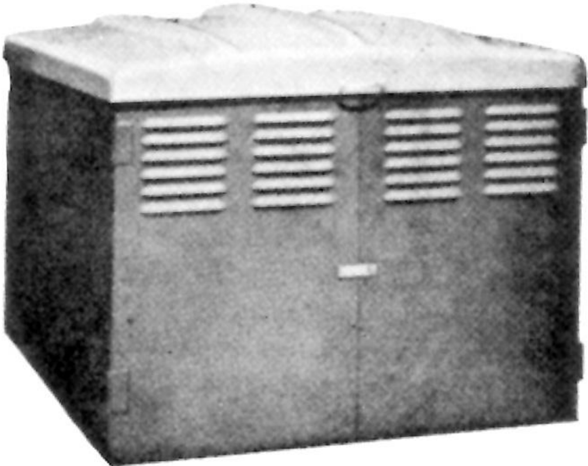
FIGURE A.8.4 (b) Closed Steel Hose House of Compact Dimensions for Installation over Private Hydrant, in Which Top Lifts Up and Doors on Front Open for Complete Accessibility.
