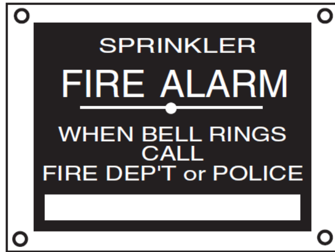
FIGURE A.8.17.1 Identification Sign.
