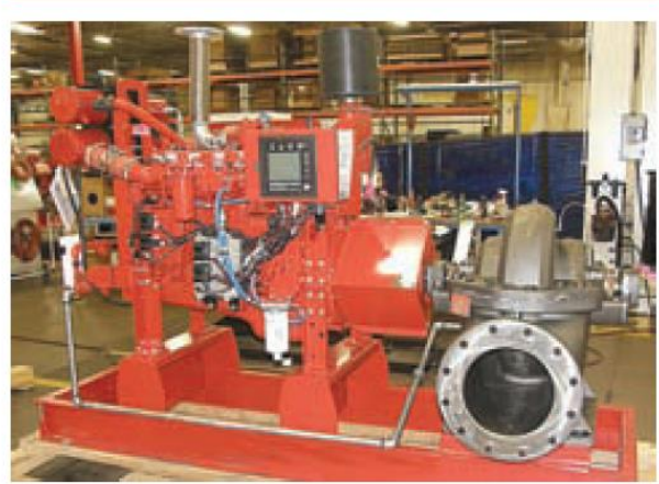
EXHIBIT II.4.8 Cooling Line for a Diesel Engine Installed Downstream of the Pump, Eliminating the Need for a Circulation Relief Valve. (Courtesy of Aon Fire Protection Engineering)
