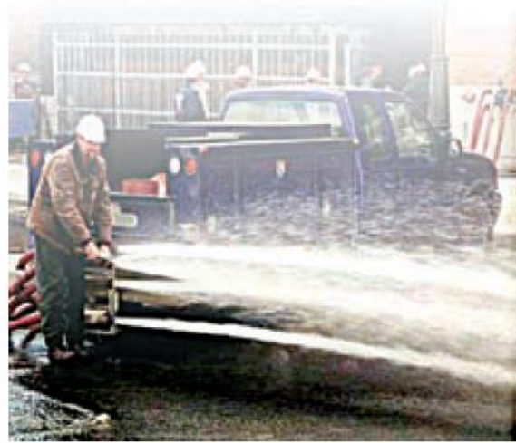
EXHIBIT II.14.8 Determining Flow Using a Pitot Gauge. (Courtesy of Underwood Fire Equipment, Inc.)
