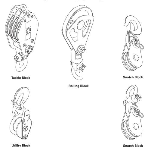
Fig. 26-5.1.1-1 Rigging Block Types
