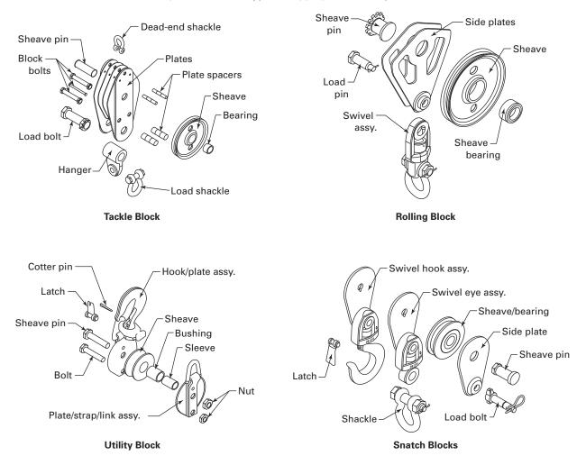
Fig. 26-5.1.1-2 Typical Rigging Block Components
