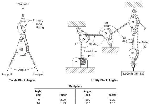
Fig. 26-5.3-1 Block Load Factor Multipliers
