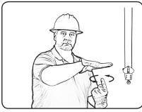
MOVE SLOWLY: Use one hand to give any motion signal and place other hand motionless in front of hand giving the motion signal. (Hoist slowly shown as example.)
