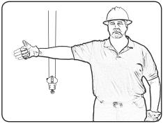
RAISE BOOM AND LOWER LOAD: With arm extended, thumb pointing upward, flex fingers in and out as long as load movement is desired.
