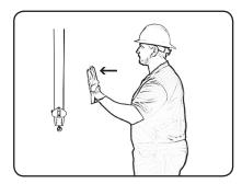
**TOWER TRAVEL:** Arm extended forward, hand open and slightly raised, make pushing motion in direction of travel.
