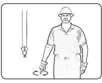
**LOWER:** With arm extended downward, forefinger pointing down, move hand in small horizontal circles.
