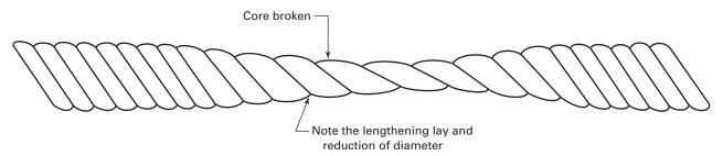
Fig. 3-2.4.2-1 Core Failure in Rotation-Resistant Rope
