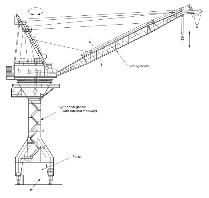
Fig. 4-0.2.1-3 Portal Crane With Luffing Boom
