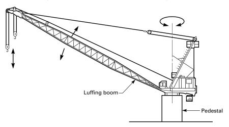
Fig. 4-0.2.1-1 Pedestal Crane With Luffing Boom
