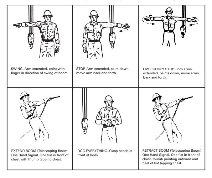
Fig. 4-3.3.4-1 Standard Hand Signals for Controlling Portal and Pedestal Cranes (Cont'd)
