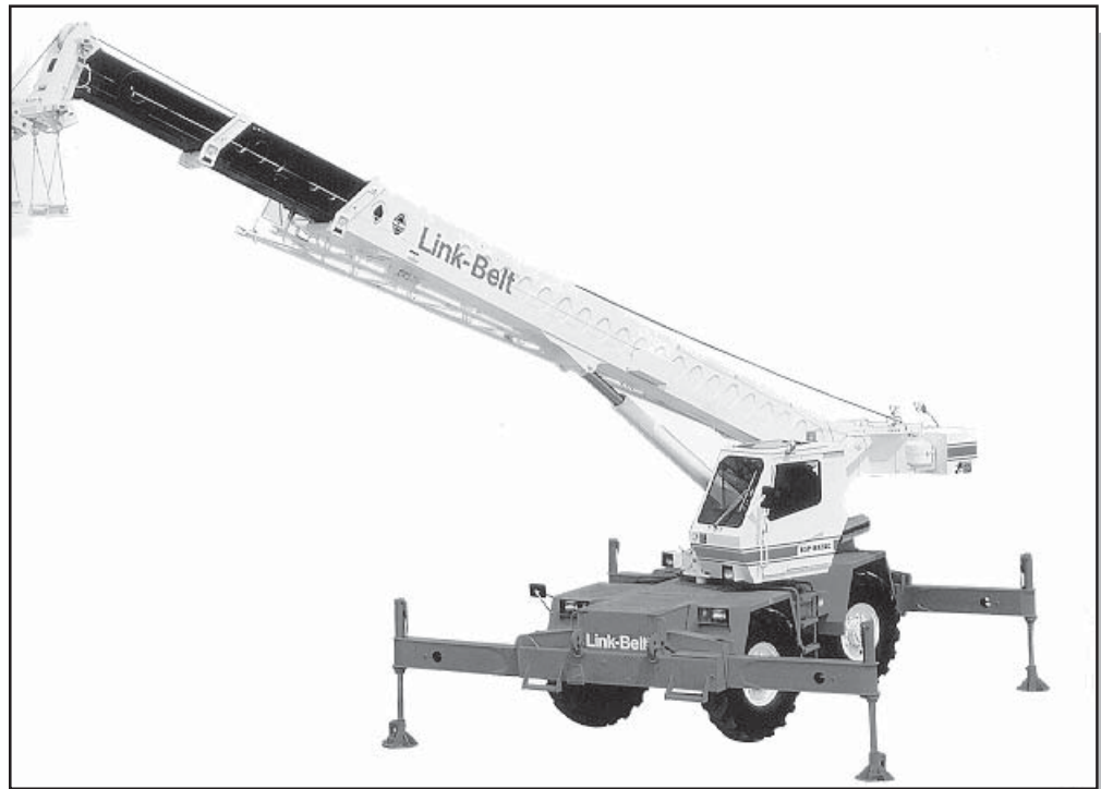
Figure 3.5-5 All Terrain Crane with Luffing
