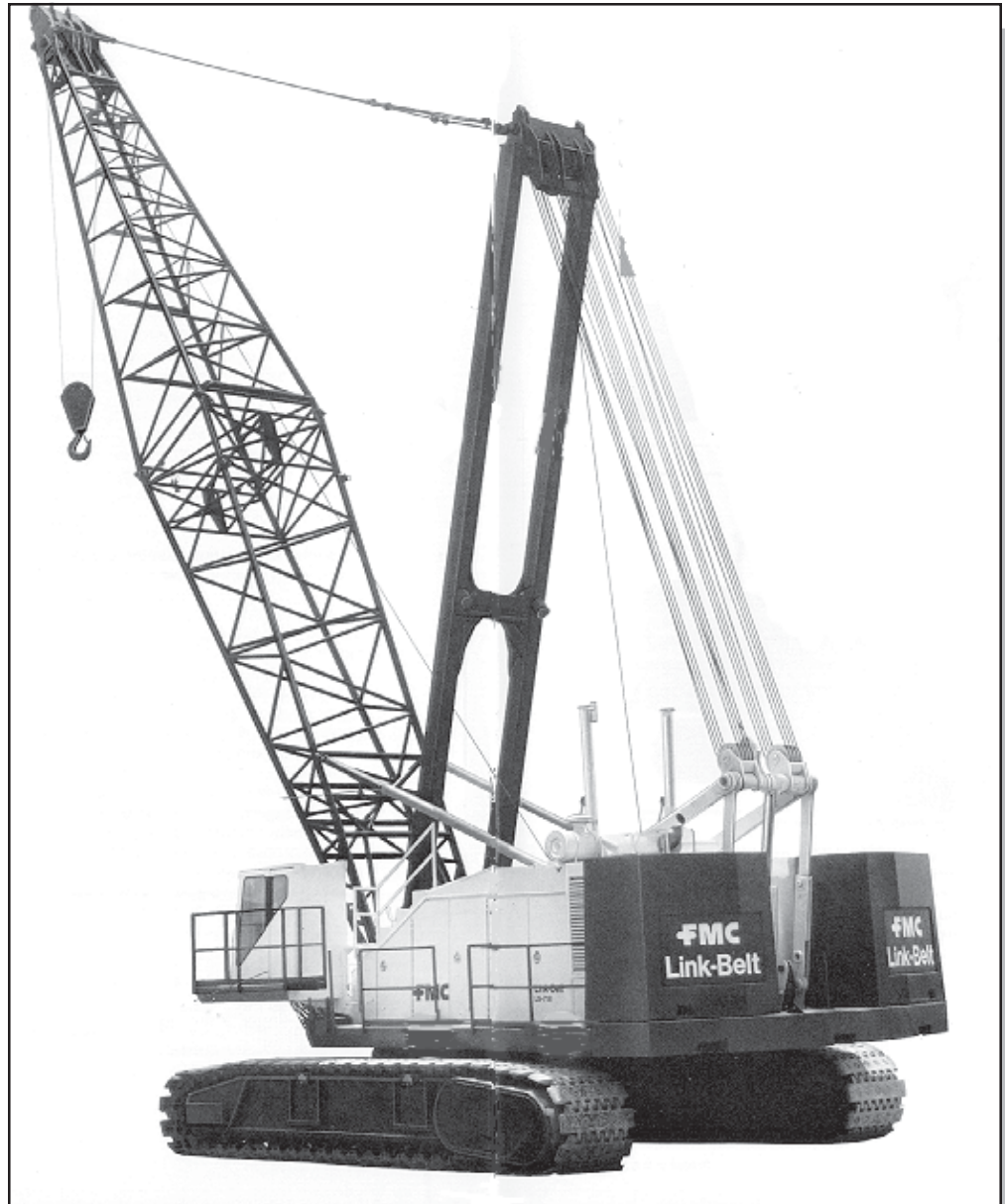
Figure 3.5-10 Lattice Boom Crawler Crane
