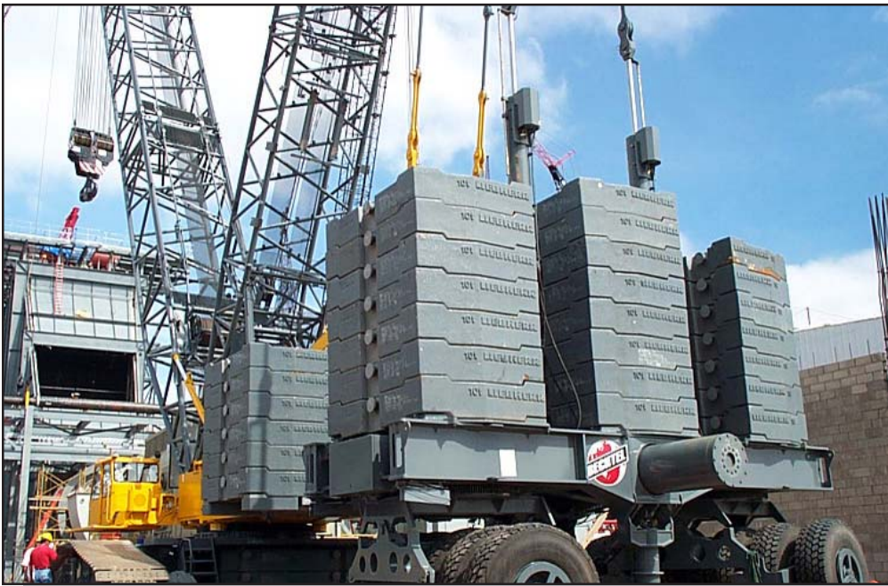
Figure 3.6-4B Super Lift Configuration of a Crawler Crane
