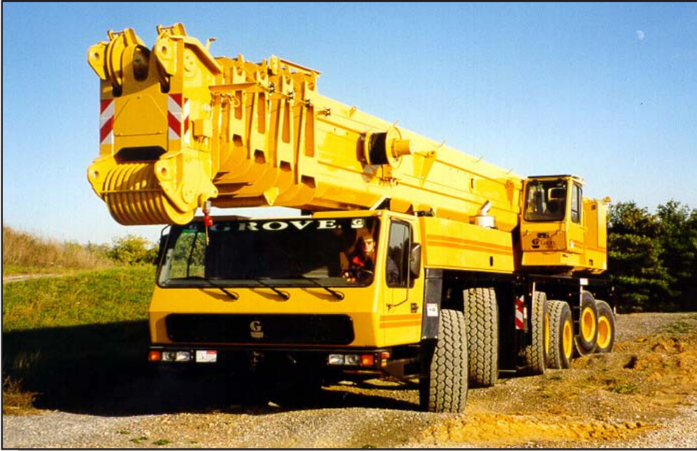
Figure 3.5-4 Al Terrain Crane
