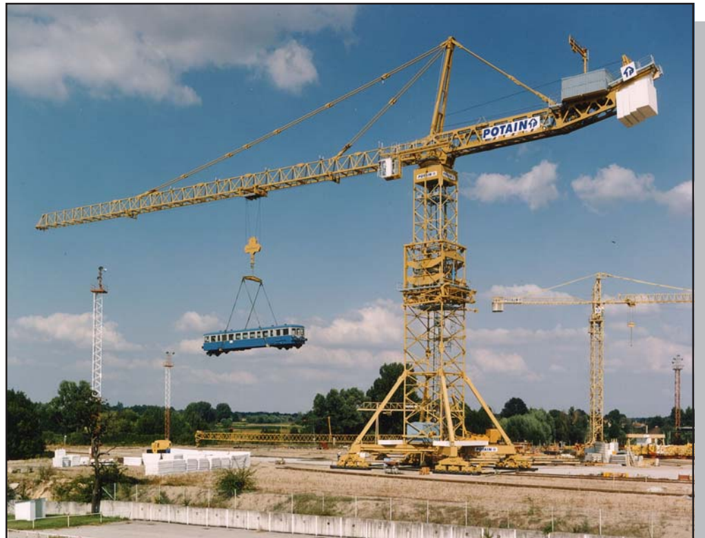
Figure 3.4-1 Horizontal Jib Tower Crane
