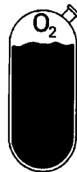
Figure 6 Oxygen is more concentrated in the vapour as propane vapour redissolves under increased pressure
