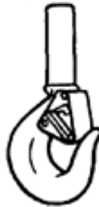
SELF-CLOSING FLAPPER LATCH (SHANK HOOK)
