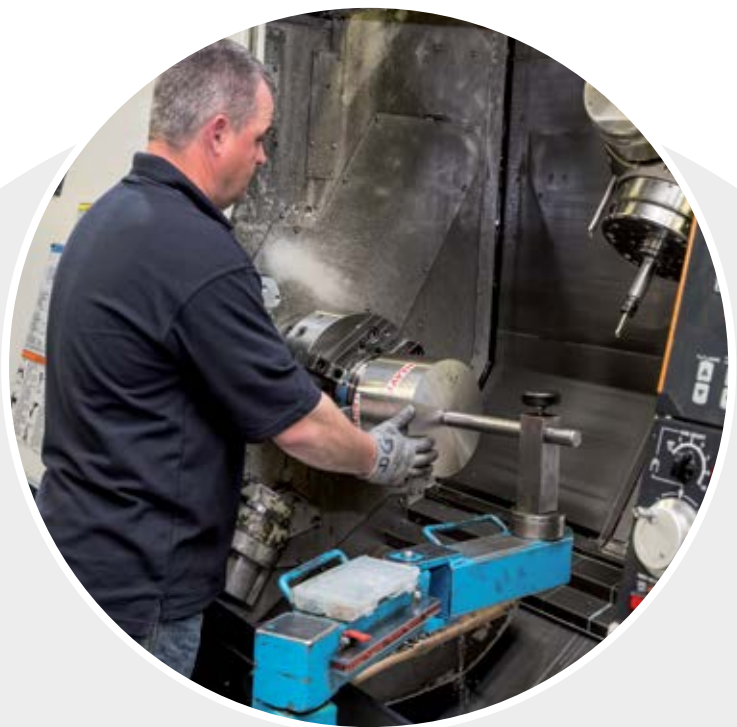
After: Operator uses custom engineered billet loader to transfer billet to CNC machine
