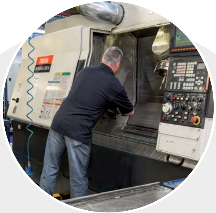
Before: Operator manually transfers the billet into the CNC machine
