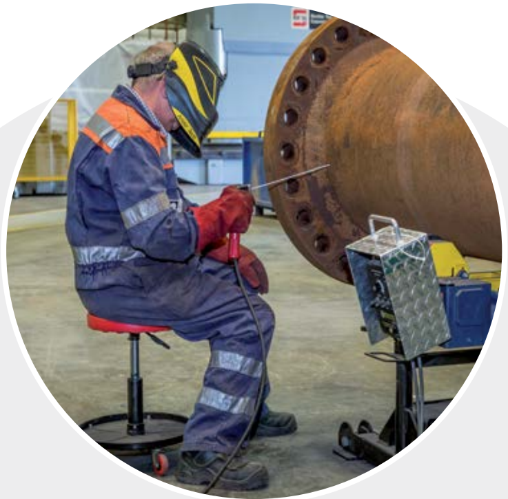
After: The use of the new roller system allows operators to alternate posture from standing to sitting during welding.
