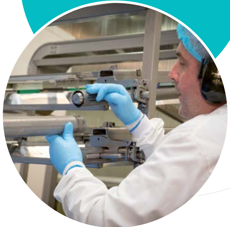
After: Operative Releases Clips to Allow the Transfer of the Positioner Head
