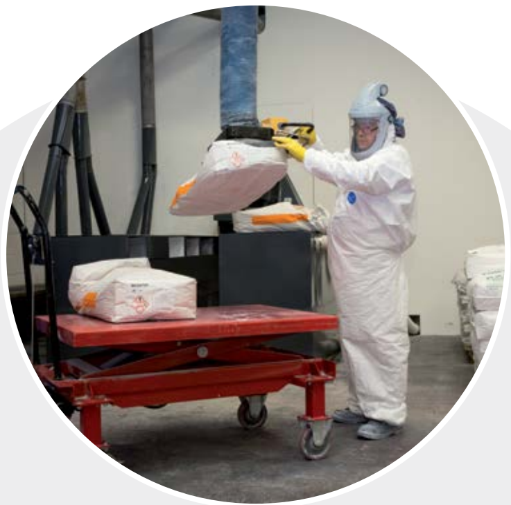
After: Operative uses a power vacuum lifter to move bag
