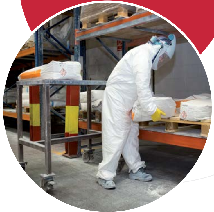
Before: Operative lifts bag manually from a storage location in the pre-mix areas and places it onto a trolley
