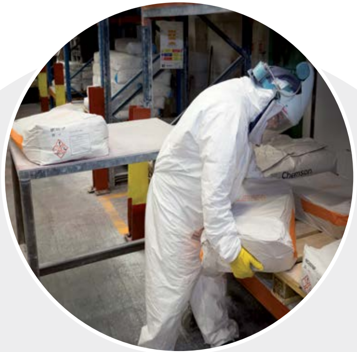
Before: Operative lifts bag and places it onto a trolley and then lifts bag from the trolley into a weigh station
