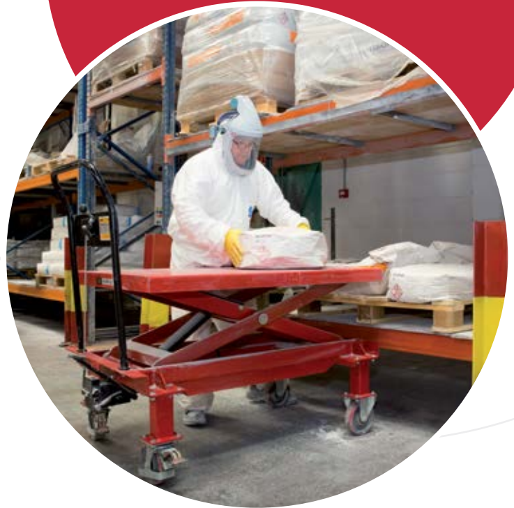
After: Operative slides bag onto a scissor lift table
