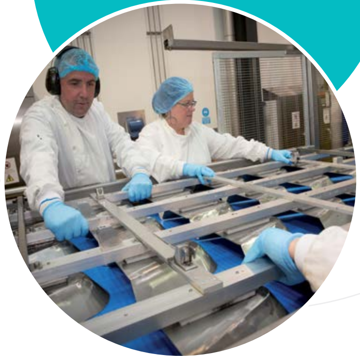
Before: Team lift by three operatives to transfer Positioner Head
