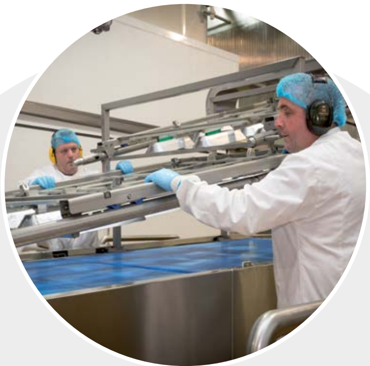
After: Rolling System allows Positioner Head to roll onto the line
