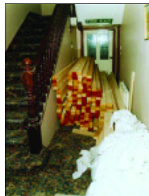
Figure 9: A blocked corridor with incorrect signage
