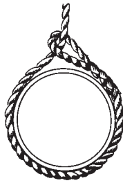
Bad Cutting Action of Wire Rope Sling Eye on Running Line
