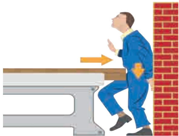
Crushing - the person is crushed between the moving object and the wall
