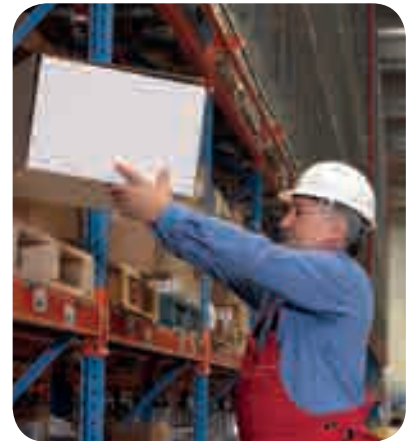
Holding a load away from your torso when lifting increases risk of injury
