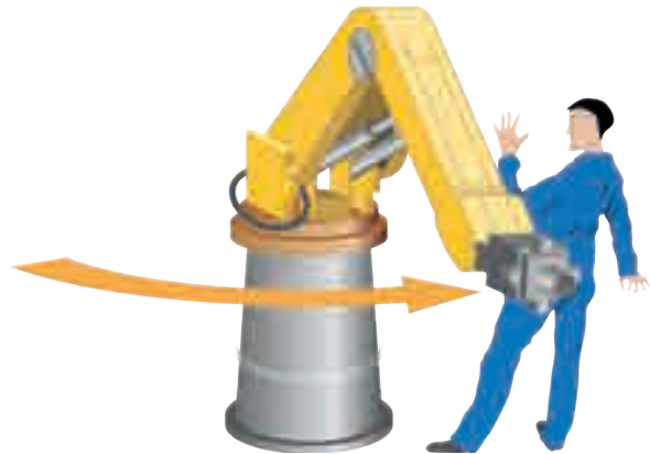
Impact - the person is struck hard by the heavy and fast-moving industrial robot
