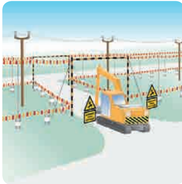
Diagram showing use of barriers, bunting and goal-posts to control proximity of plant to overhead power lines (Based on original source HSG144 The safe use of vehicles on construction sites (2nd ed.), HSE, 2009 ( www.hse.gov.uk/pubns/priced/hsg144.pdf ))
