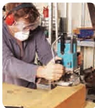
A worker wearing a filtering facepiece respirator to prevent inhalation of wood dust
