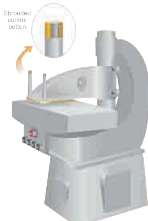
Two-hand controls on a click press; the operator is at risk of a crushing injury if the press operates when their hand is between the top and bottom plates
