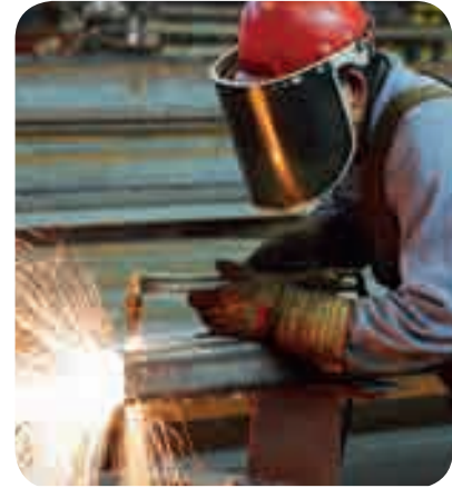
Workwear and PPE covers all exposed skin, with a dark visor to protect the face and eyes from UV, visible and IR radiations generated during oxy-acetylene cutting
