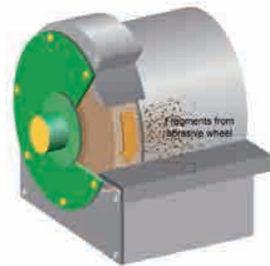
Stabbing or puncture - small fragments of the abrasive wheel are ejected at high speed and can cause penetration injury, particularly to the eyes
