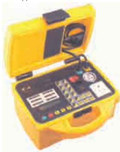
A portable appliance test meter
