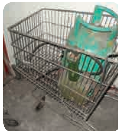
Unsafe storage of gas cylinders
