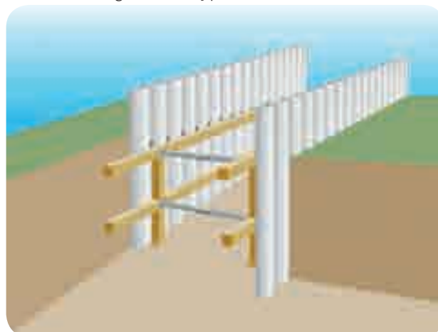
Shoring the sides of an excavation by 'close sheeting'
