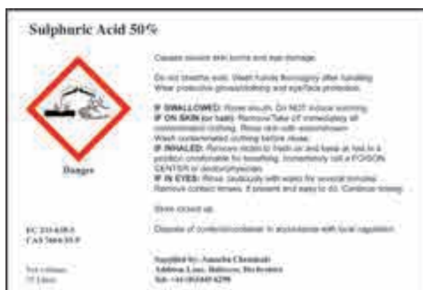
A label showing the key information about the hazardous nature of the product
