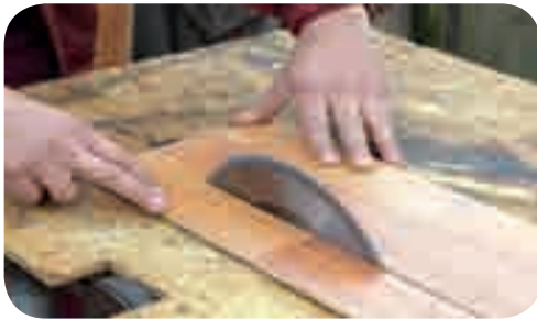
Machine being used without the appropriate guard
