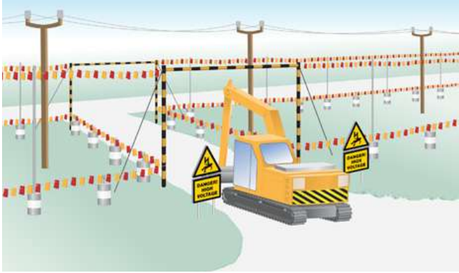
Diagram showing use of barriers, bunting and goal-posts to control proximity of plant to overhead power lines 2nd ed.), The safe use of vehicles on construction sites Based on original source HSG144 (pdf.http://www.hse.gov.uk/pubns/priced/hsg144) 2009 ,HSE
