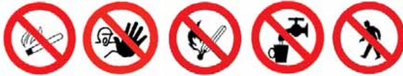
It is prohibited to smoke Entry prohibited to unauthorised persons It is prohibited to smoke and light fires Water not suitable for drinking Access by pedestrians is prohibited
