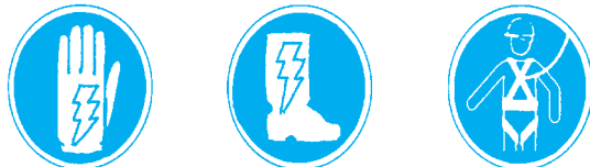
It is compulsory to wear insulated gloves It is compulsory to wear insulated boots It is compulsory to wear a safety belt
