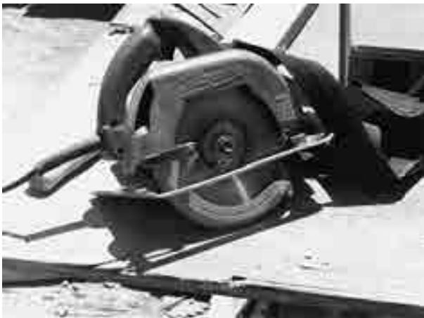
FIGURE 8.16 Circular saw with blade guard and equipped with a constant pressure switch
