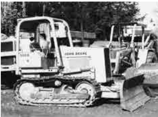
FIGURE 8.29 Dozer with rollover protection and overhead protection
