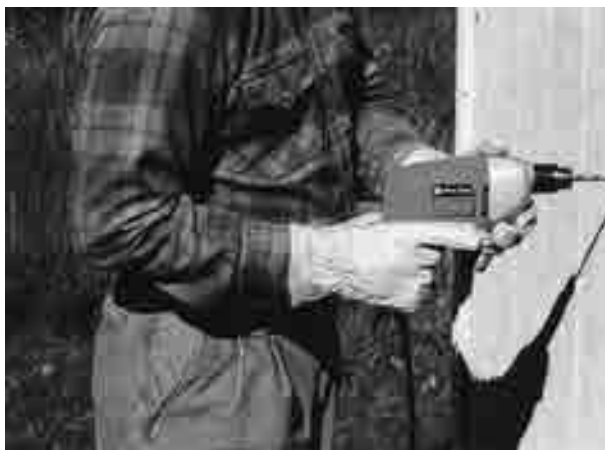
FIGURE 11.18 A worker with a 90° bend of arm and a straight wrist is in a neutral position
