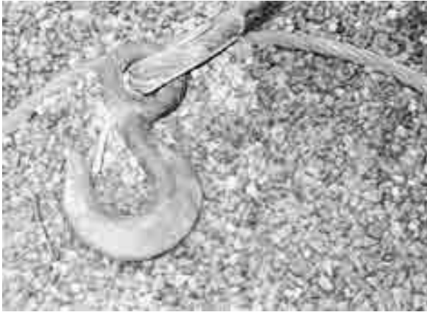
FIGURE 8.28 Example of a hook with a safety latch
