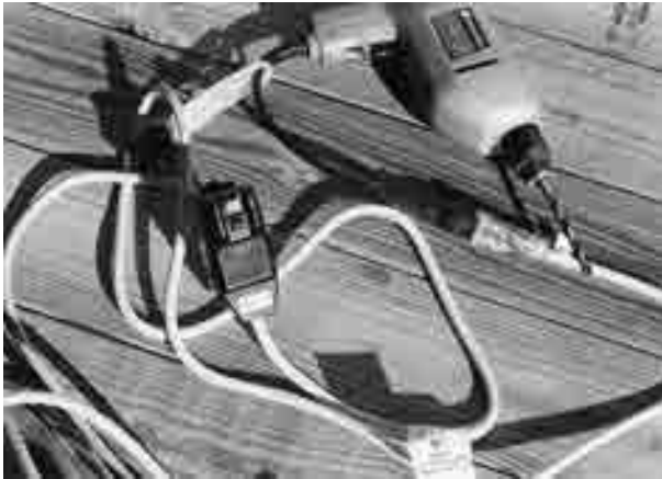
FIGURE 7.26 Example of a ground-fault circuit interrupter connected to a drill
