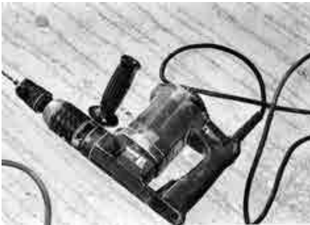
FIGURE 11.20 Typical power tool which can be used with either hand by changing the handle and also using both hands to prevent torquing
