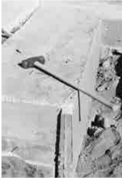
FIGURE 7.55 Wooden handled sledge hammer in good repair
