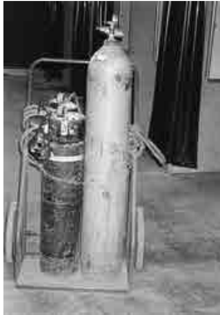
FIGURE 7.9 Compressed gas welding set up with chain-secured gas cylinders
