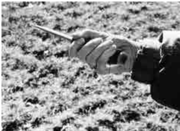
FIGURE 11.19 A handle on a screwdriver which fits the individual’s hand and prevents soft tissue injuries
