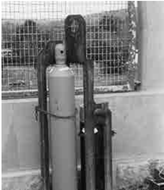
FIGURE 7.8 Cradle for lifting compressed gas cylinders
