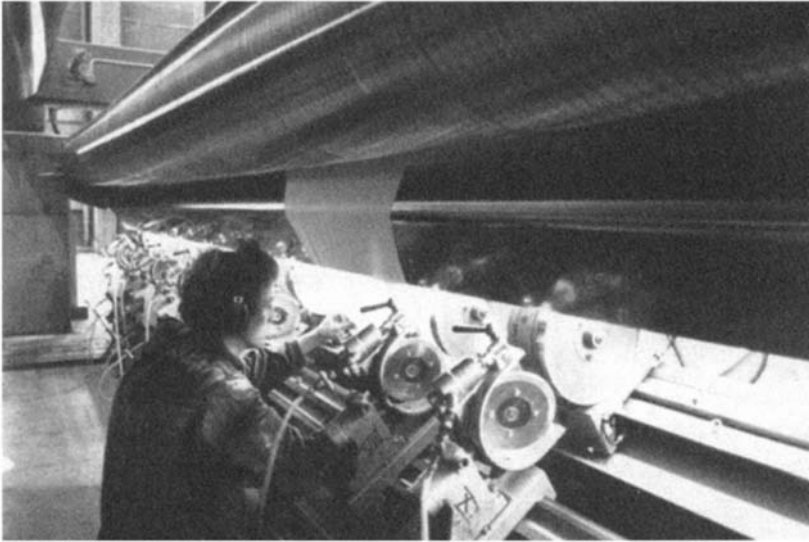
Figure 7.5. A new sheet of paper is drawn towards the reel cutters of a paper-rolling machine.
