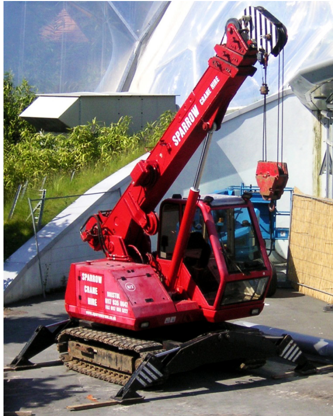
Figure 6.21: Telescopic mobile crane Mini crane/crawler tracks/outriggers in use
