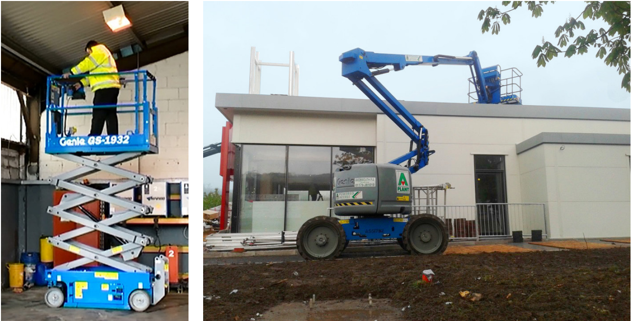
Figure 8.17: MEWPs – Self-propelled scissors lift and articulated boom
