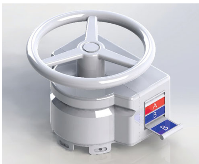
Figure 10.3 Valve open – key A free, key B trapped Source: ISS Safety Ltd.
