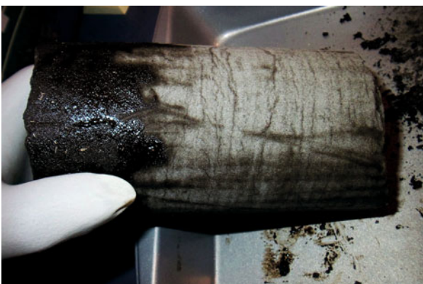
Figure 10.4 Example of a hydrate ice plug Source: US Department of Energy.
