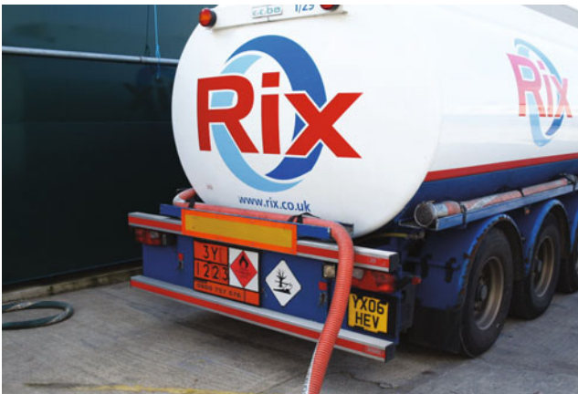
Figure 20.3 Hazard signboard on rear of tanker Source: Wise Global Training.
