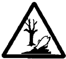
Dangerous to the environment
