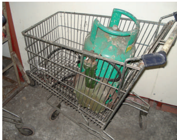
Unsafe storage of gas cylinders
