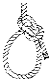
Illustration #161 - Knots = 50% Efficiency
