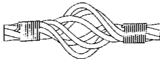
Illustration #25 - Wire Rope Bird Caging
