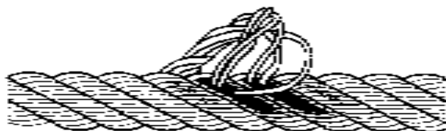
Illustration #26 – Wire Rope Protruding Core
