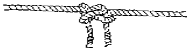
Illustration #162 - Bend = 50% Efficiency
