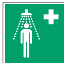
E012: Safety shower
