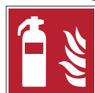
F001: Fire extinguisher
