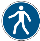
M024: Use this walkway
