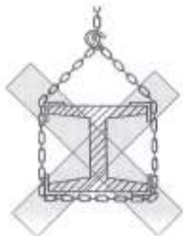
Bad practice – packing ineffective chain links may be bent
