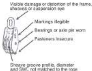
Figure 15 Pulley Block Inspection Points
