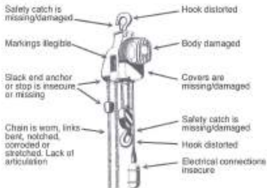
Figure 11 Power Operated Chain Block Inspection Points
