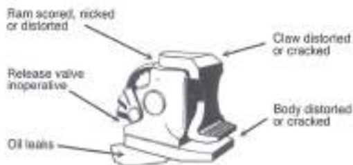
Figure 23 Hydraulic Jack Inspection Points
