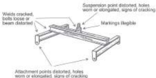
Figure 36 Lifting Beam and Spreader Inspection Points
