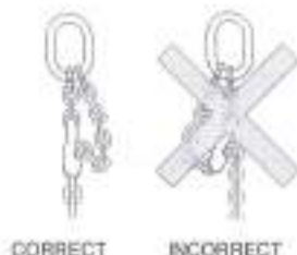
Figure 25 Correct and Incorrect Use of a Chain Clutch
