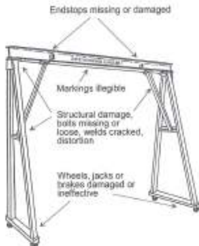
Figure 22 Mobile Gantry Inspection Points
