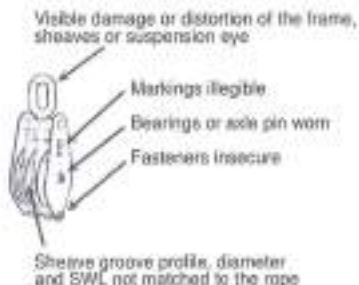
Figure 8 Pulley Block Inspection Points
