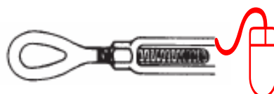
Fig. 7 Incorrect (No Lock Wire)
