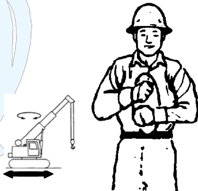
Fig. 17 TRAVEL (Both Tracks) . Use both fists in front of body, making a circular motion about each other, indicating direction of travel, forward or backward. (For land crane only)
