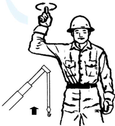
Fig. 1 HOIST. With forearm vertical, forefinger pointing up, move hand in small horizontal circle
