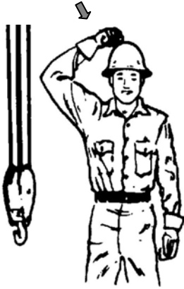
Fig. 3 USE MAIN HOIST. Tap fist on head; then use regular signals
