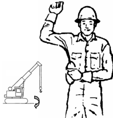
Fig. 18 TRAVEL (One Tracks) . Lock on side indicated by raised fist. Travel opposite track in direction indicated by circular motion of other fist, rotated vertically in front of body. (For land crane only)
