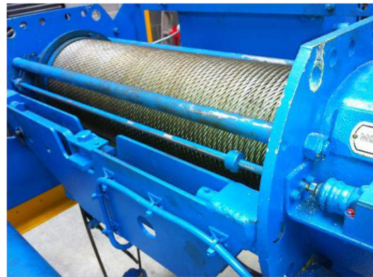
Wire rope drum used to accommodate the load rope on a typical electric wire rope hoist
