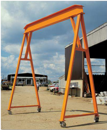
Internally Braced Gantry
