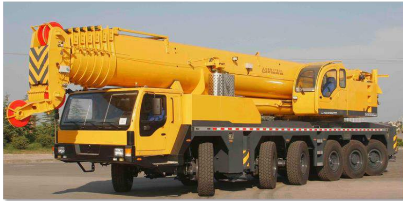
All Terrain Crane
