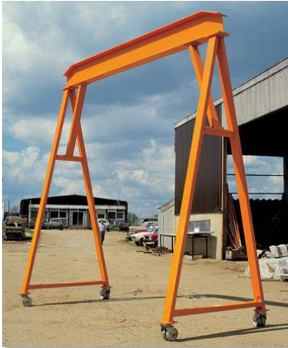
Internally Braced Gantry
