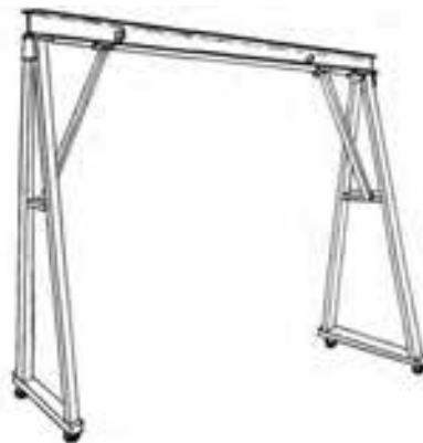
Figure 12.8 'A' frame gantry
