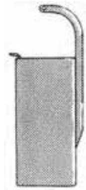
Figure 3.5 Typical load chain collecting box
