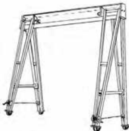
Figure 12.11 Self erecting gantry
