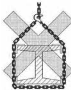
Figure 1A5.22 Bad practice - packing ineffective chain links may be bent
