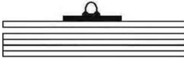
Figure 27.10 Vacuum lifter used to remove one plate or sheet from a stack
