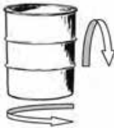
Figure 24.5 Side gripping barrel lifters provide rotation about both axis
