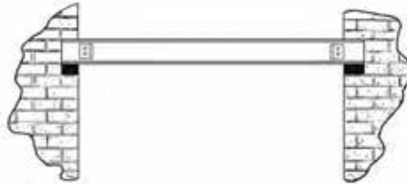
Figure 11.2 Runway built in each end (encastre)
