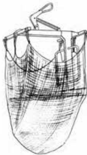
Figure 25.2 Crane fork fitted with a safety net to retain any part of the load inadvertently released
