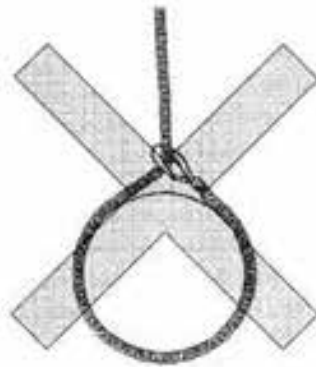
Never hook back a load chain like this
