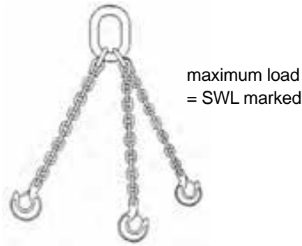
Figure 14.26 Three leg sling in straight lift
