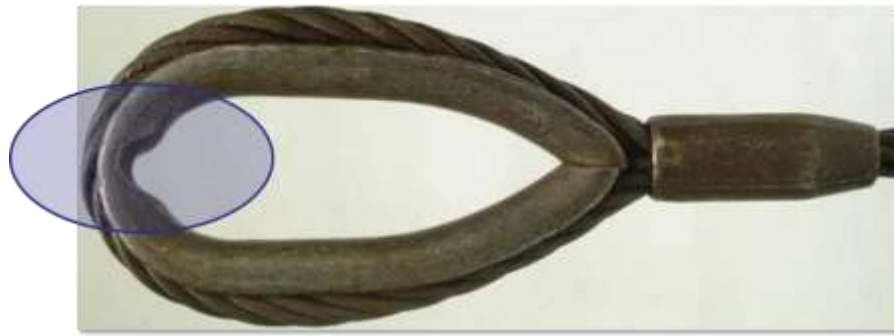
Damaged Reeving Thimble
