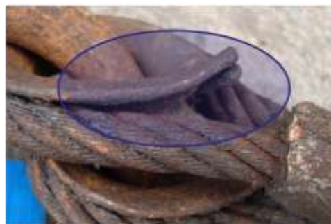
Damaged Ferrule (Side Loading)
