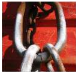
Cracked Master Link
