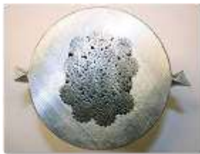
Cross- Section of a Pressed Ferrule Termination
