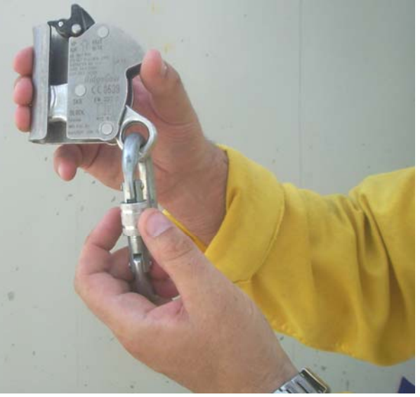
Check yellow side to ensure That inspection has been carried out in the last 7 days
