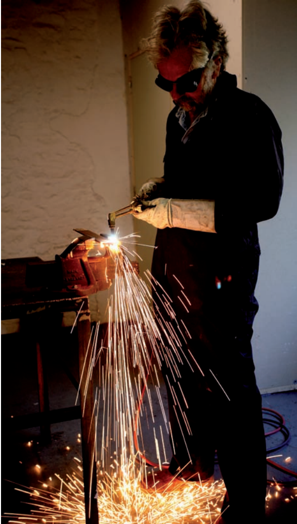
Sparks from welding or burning is a common ignition source
