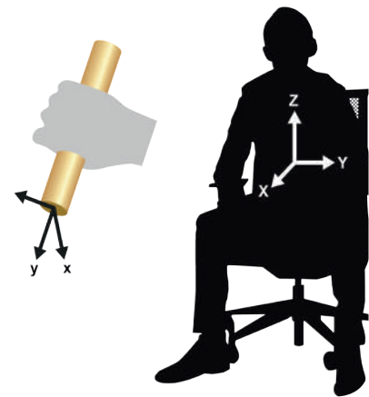
Axes of vibration for hand-transmitted and whole-body vibration
