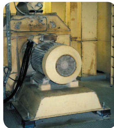
Anti-vibration mounts isolate grinder from supporting surface
