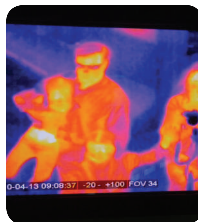
Image displayed by an infrared camera sensitive to IR radiation given off by the human body
