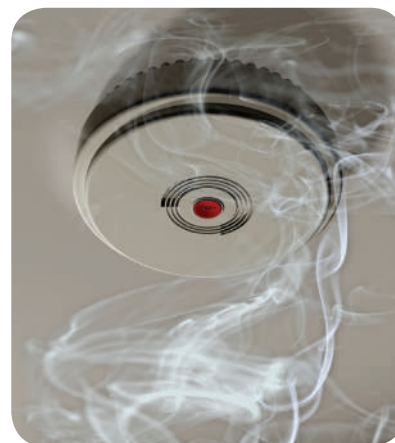
Smoke detector Contains an encapsulated radionuclide - americium 241
