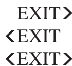
FIGURE A.7.10.6.2 Directional Indicators.
