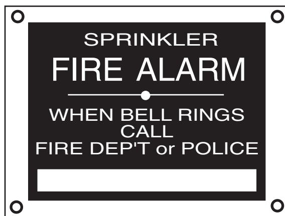
FIGURE A.8.17.1 Identification Sign.
