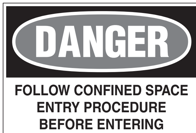
FIGURE A.4.7.2 Confined Space Entry Sign.
