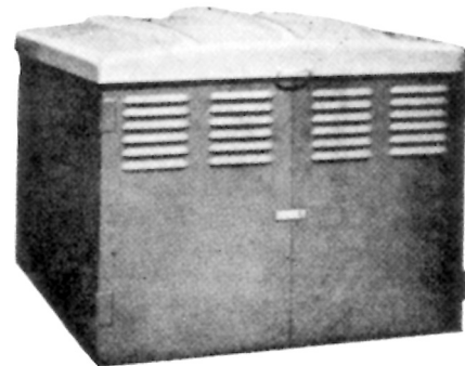
FIGURE A.8.4(b) Closed Steel Hose House of Compact Dimensions for Installation over a Private Hydrant, in Which Top Lifts Up and Doors on Front Open for Complete Accessibility.
