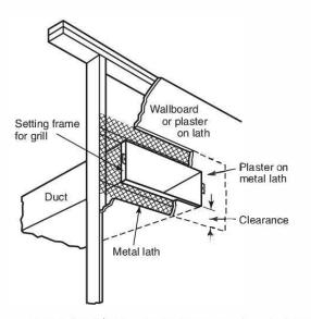
FIGURE 6.1.2.7 (a) An Arrangement for Closing Ends of Clearance Space Around a Supply Duct. A similar arrangement can be used where a duct continues through the partition.
