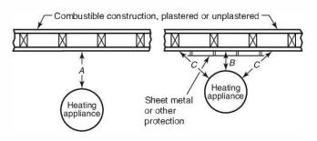
A equals the required clearance with no protection as specified in Table 6.1.2.1.
