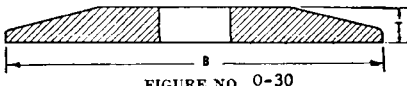
Driving flange secured to spindle for use only on portable wheels with threaded inserts or projecting studs.
