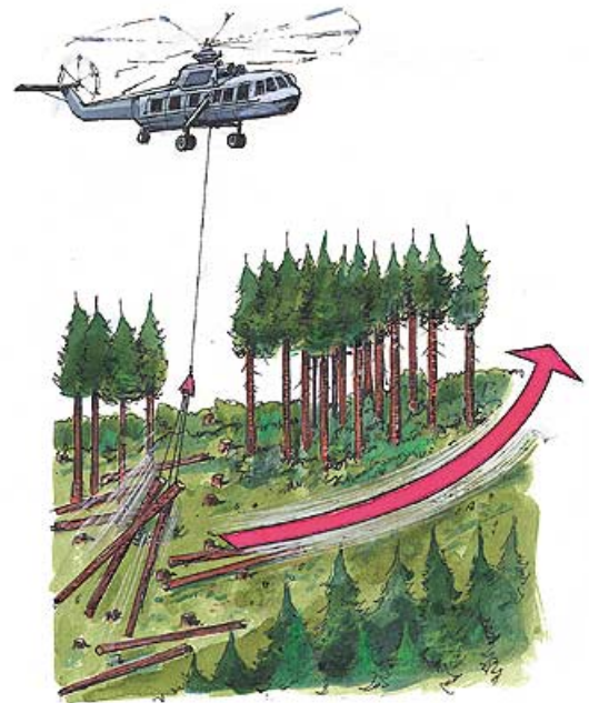
Plan turns to avoid overhead hazards and brushing of leave-trees.
