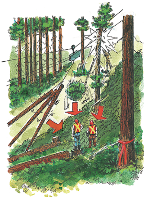
Workers must stay in safe locations to avoid overhead hazards and swinging of the log turn. These workers are not in the clear.
