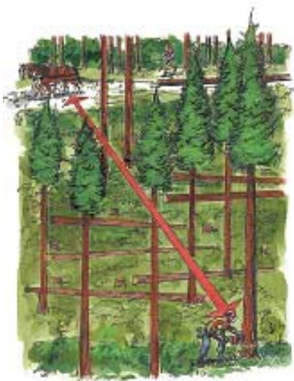
Always maintain a safe distance of at least two tree-lengths between fallers, horses and other workers.
