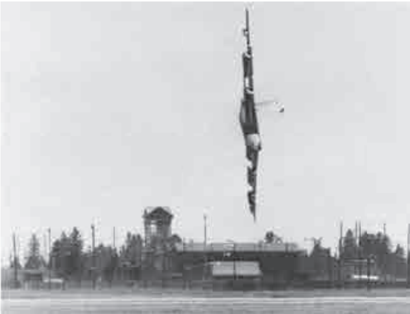
AWRY: the B-52 exceeded authorized maneuvers and, after aborting a landing, lost altitude
