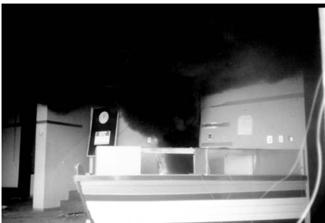
Figure 9.1 Outflow of smoke through the upper part of an opening in a compartment fire.
