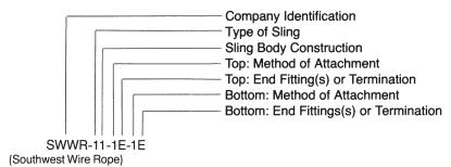
NOTE: Above example is a standard eye and eye sling, mechanically spliced.
