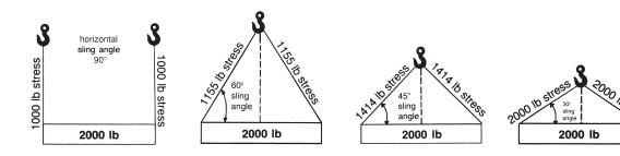
The rated capacity of a multiple leg sling is directly affected by the angle of the sling leg with the horizontal. As this angle decreases, the stress on each leg increases with the same load. If the sling angle is known, the capacity can be readily determined by multiplying the sling's vertical capacity by the appropriate load angle factor from the table at right.
