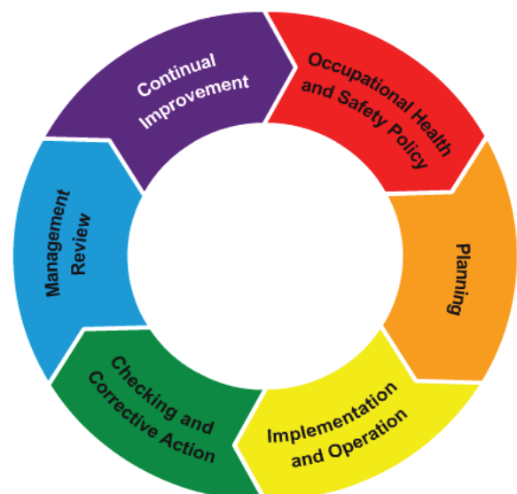
Occupational Health and Safety Assessment Series 18001 (OHSAS 18001): health and safety management model
