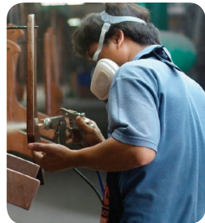
Worker being exposed to airborne contaminant
