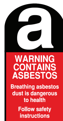
Example of an asbestos warning label
