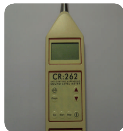
An Integrating Sound Level Meter (ISLM)
